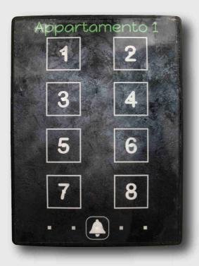
A touch-sensitive numeric keypad controls the opening of both the **outer gate** and the entrance door of each individual **apartment**.
